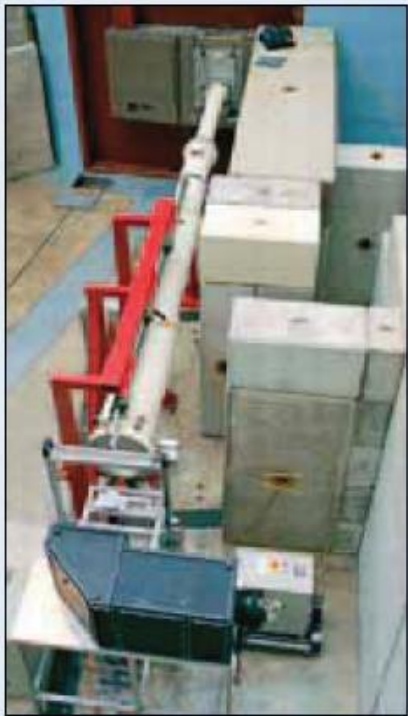
Internal view of NEUTRA (shielding partially removed). Right: graphic representation of NEUTRA.
