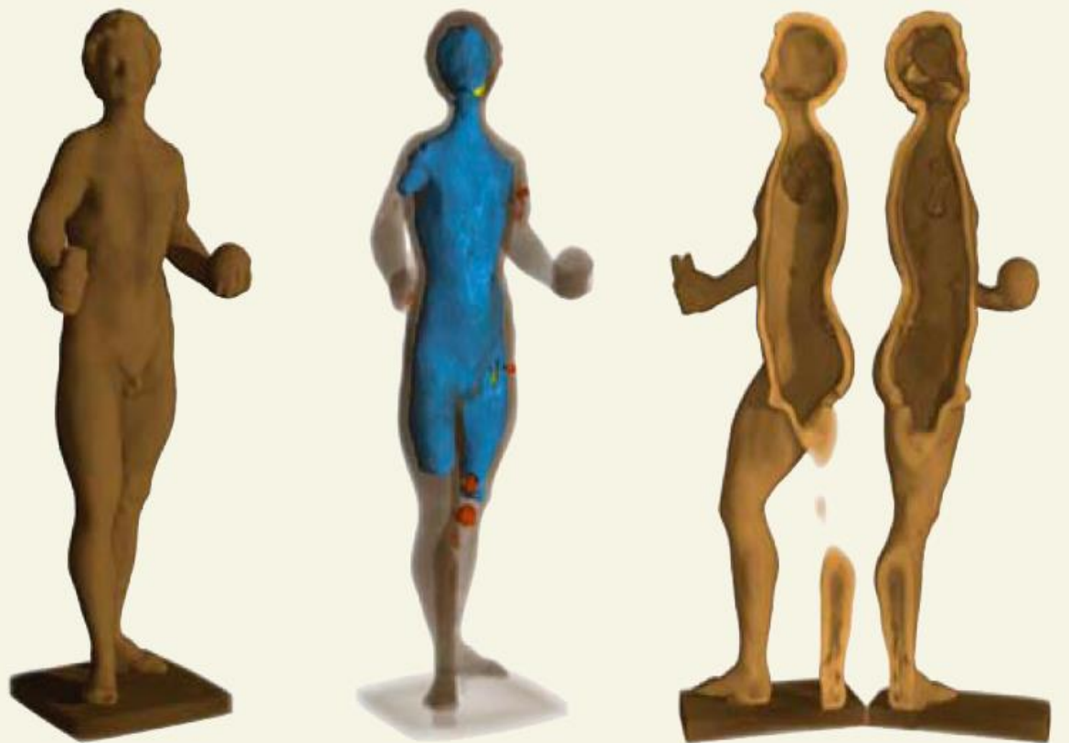
Figure 24: Tomographic views of a bronze sculpture: virtual slices can be created without damaging this unique object.
