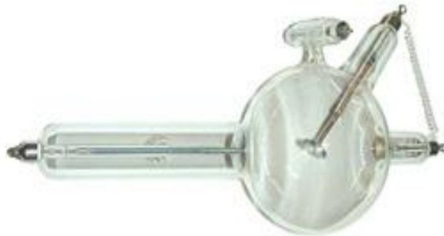
Schematic diagram of a therapy x-ray tube with hooded anode.
